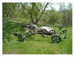
This image of a cart-borne system shows a simple 2 sensor array in operation.
