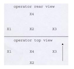
Sensor X4 is located at a different level than the other sensors in order to derive the 3D vertical gradient. Output values are determined automatically using the GEM system console.
