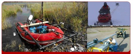
Multi-sensor configurations can be implemented on various platforms. These platforms take advantage of GEM's 4-channel "true simultaneous" capabilities
